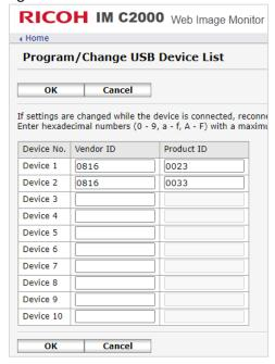
In User Tools > Machine Features, go to System Settings as MFP admin, Networ/Interface and External Interface Software Settings.
