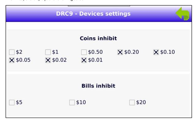
A coin or a bill is rejected by checking the box at the right of the value to inhibit.
