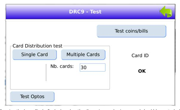
Pressing the key « Single Card » launches the dispensing mechanism, a card should be unstacked from the feeder and should drop in the dispensing basket.
