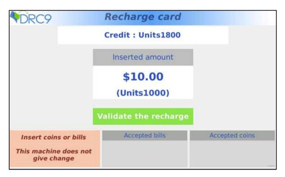
The user will have to press key « Validate the recharge » for completing the recharging transaction. In case the user does not press this key, a transaction of end is launched automatically after 20 seconds of inactivity.
